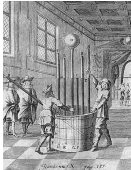
Figure 6: Drawing illustrating that the size and volume above the mercury does not influence the height of the mercury column.
