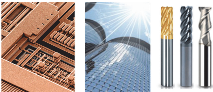
Figure 1. (Left) Copper interconnect metallization (~109 connections) in a transistor, courtesy of IBM, 1997. Bus bar (metallic frame) in lower part is ~20 \mu\text{m} wide, about 1/5 the size of human hair (average diameter ~100 \mu\text{m} ). Colorized SEM view after removal of insulating layers by chemical etching. http://www-03.ibm.com/ibm/history/ibm100/us/en/icons/copperchip/ . (Middle) Coated architectural glass in office buildings. Figure courtesy of Hy-Power Nano Inc. Brampton, Ontario, Canada. (Right) TiN, TiAlN, and TiB 2 (left to right) coated tools. Figure courtesy of SGS Tool Company. Munroe Falls, Ohio, USA.
