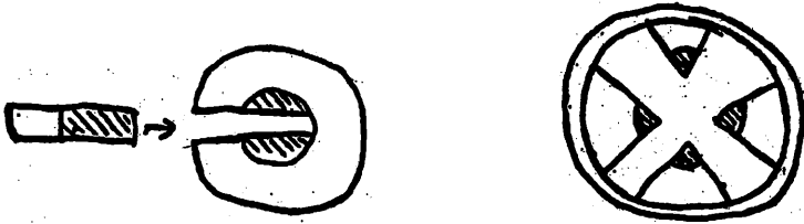
Fig.8: Schematic representation of the two types of atomic bombs, such as they were presented in the "Los Alamos Primer". Left: the "gun" type, right the "implosion" type.
