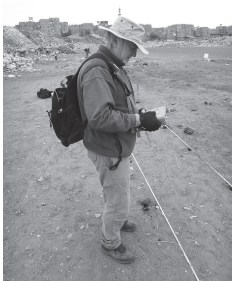
Figure 9: Electrical resistivity sounding is based on the estimation of the electrical conductivity or resistivity of the soil (source: M. De Dapper).
