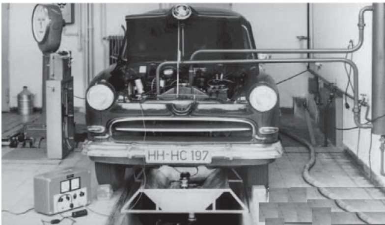
Figure 3.2: Shell PAE Laboratory Hamburg in 1956, with a Ford Taunus on the first roller dynamometer.
