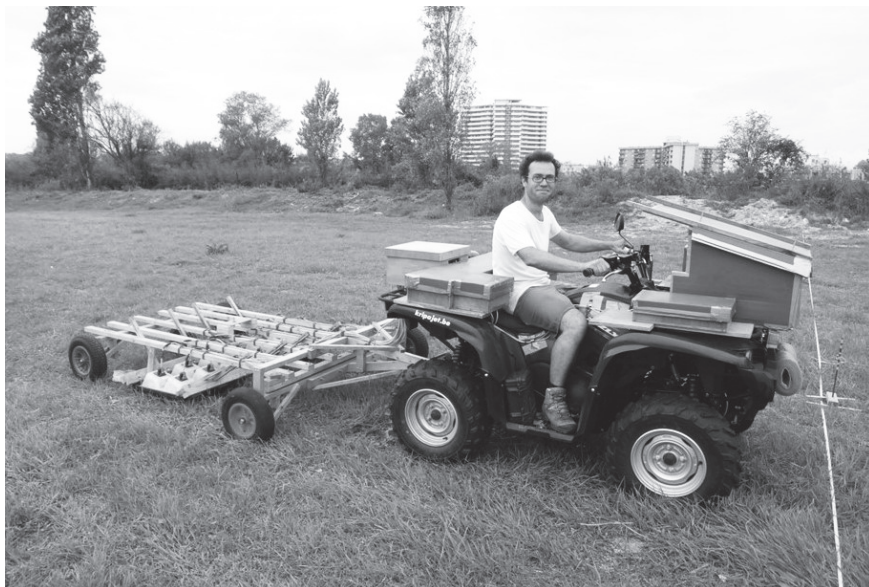
Figure 7: GPR uses radar pulses to image the subsurface (source: M. De Dapper).
