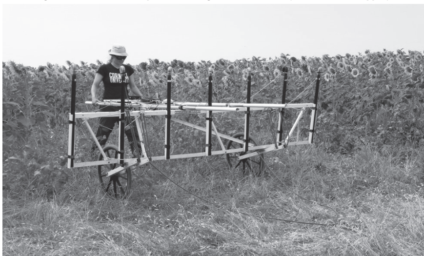
Figure 8: Magnetometry detects variations of the Earth's geomagnetic field (source: M. De Dapper).
