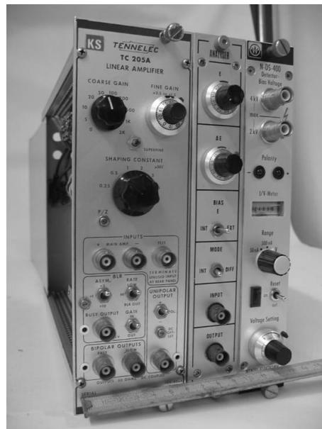
Figure 15. NIM-modules: shaping amplifier with P/Z and BLR (TENNELEC, USA), SCA-discriminator (Nuclear Enterprises, UK) and 4 kV bias power supply for semiconductor detectors (Wenzel, D)
