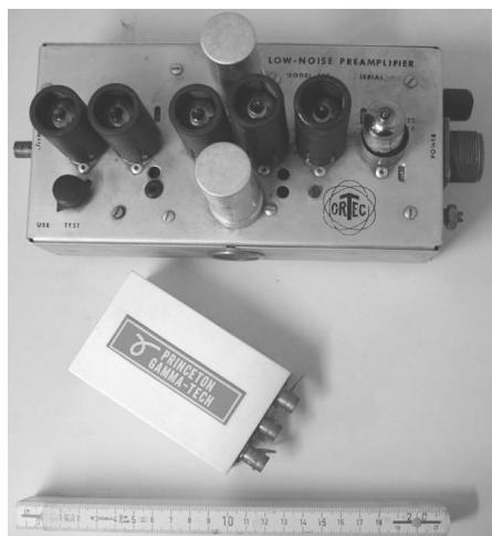
Figure 14. Top: low-noise preamplifier model 103 for semiconductor detectors with 6 vacuum tubes by ORTEC (Oak Ridge, TN, USA) 1969
