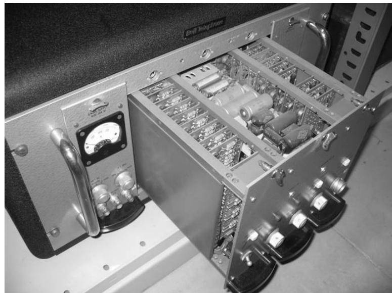
Figure 13. Early modular nuclear instrumentation with germanium transistors by Bell Telephone Hoboken-Antwerp (1962). It contains a high voltage power supply for Geiger-Müller counters and a control unit for an angular correlation measurement set-up
