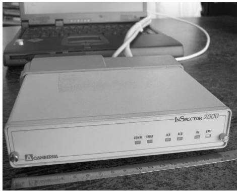
Figure 19. Portable spectroscopy workstation, model InSpector 2000 by Canberra Ind. (Meriden, CT, USA). This completely integrated high resolution measuring chain for Ge-detector is fully digitally controlled by a notebook PC via USB. It has 10 hours autonomy of on a standard camcorder battery pack
