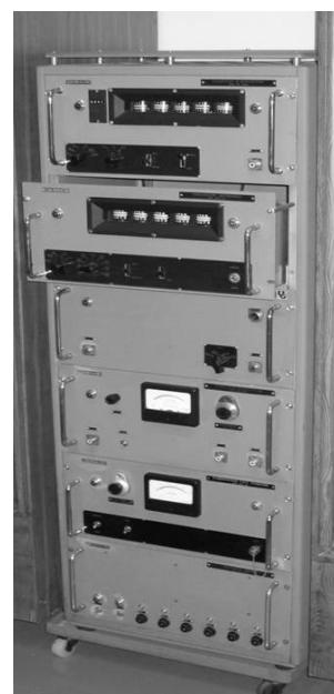
Figure 10 (right). MBLE spectrometer: Single Channel Analyser with pulse amplifier, discriminator, scalers and power supply, all with vacuum tubes (150x50x40cm<sup>3</sup>)
