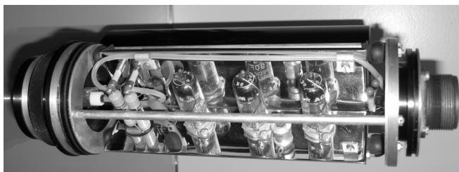
Figure 11. MBLE preamplifier PNB 015 for scintillation detector with 3 SQ E90F tubes
