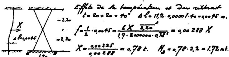
Fig. 3 Vessy Bridge calculations for the X-shaped cross walls.
