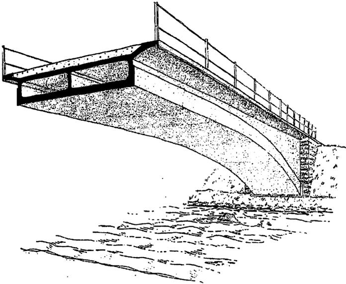
Fig.11 Hollow box, three-hinged arch bridge at Zuoz.
