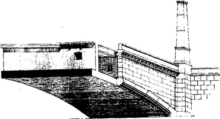
Fig.10 Stauffacher Bridge with a heavy arch that supports the crosswalls and deck as well as the masonry wall façade.
